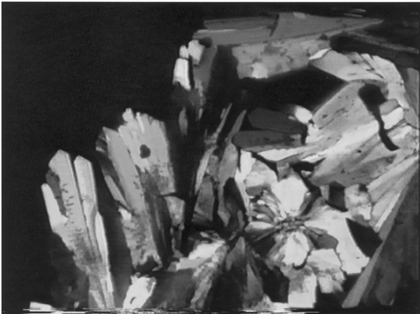
Fig. 7. Needle crystals after transformation and melting of spherulites (180°C). Image width equivalent to 2 mm.
