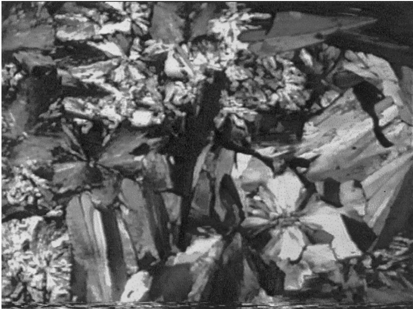
Fig. 6. Transformation of spherulites to needles (150°C). Image width equivalent to 2 mm.
